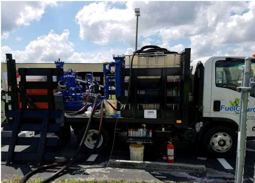
“Blue Bolt” Customized filtration equipment mounted on stake-body truck.
